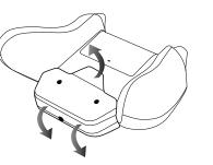
To remove the Audio Controller, apply gentle downward pressure to disengage the tab on the bottom of the controller.
