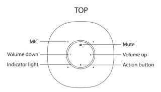
Note: the volume up/down button is only for adjusting Alexa sound.
