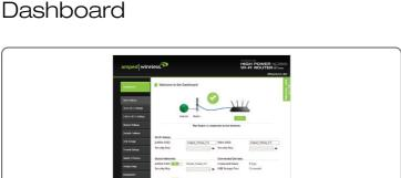
Once you have completed the Setup Wizard, you will now see the Dashboard when you access http://setup.ampedwireless.com. You will not see the Setup Wizard again. Through the Dashboard you can further adjust settings and access the features of the Router. Here you will find features like
