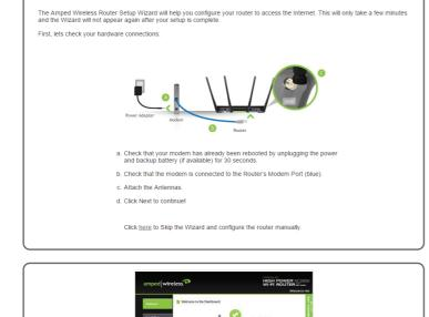
Double check that the modem is connected to the Router's Modem port.
