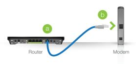
Make sure the included Ethernet cable is connected to the Modem port on your Router. Connect the other end of the cable to your Modem.
