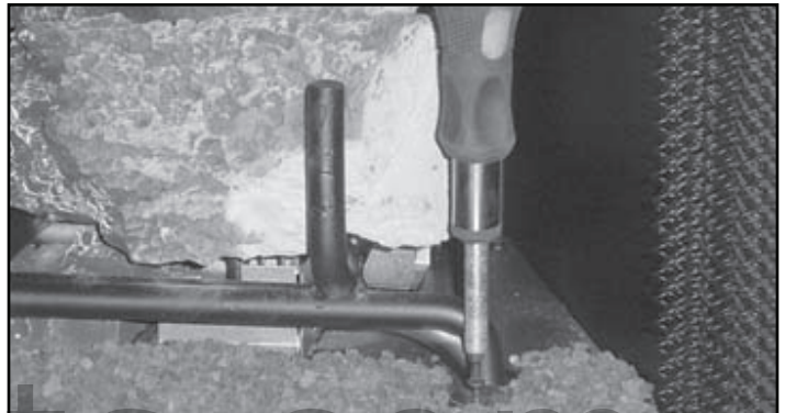
Figure 12.8 Remove Screws from Sides
