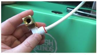
27. Connect new John Guest elbow to new rinse nozzle stem. Be careful not to damage plastic wing nut. Make sure to install red retaining clips.
