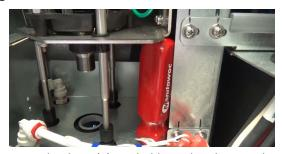
7. Loosen the three (3) cup holder rods. Pliers can be used at top of rods if needed.
