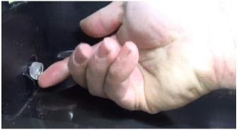
NOTE: New nozzle should be installed with thickest part of plastic at top so spray cutout faces down into basin.
