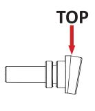
32. Install new nozzle and connect retaining clip to outside of basin. Make sure o-ring is inside basin.
