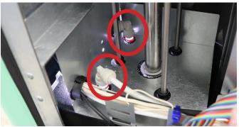
NOTE: May need to disconnect farthest John Guest Fitting from water line to get fitting over stem. Access hole in front of unit can be used to remove the retaining clip and fitting.
