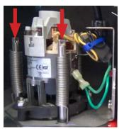
NOTE: It may be helpful to prop up the blender motor plate using end of universal screwdriver.
