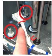
18. Hold stem fitting inside unit with one hand and unscrew blender shaft rinse nozzle block with other hand. Set stem fitting and rinse nozzle block aside. Repeat for other blender shaft rinse block and stem fitting.
