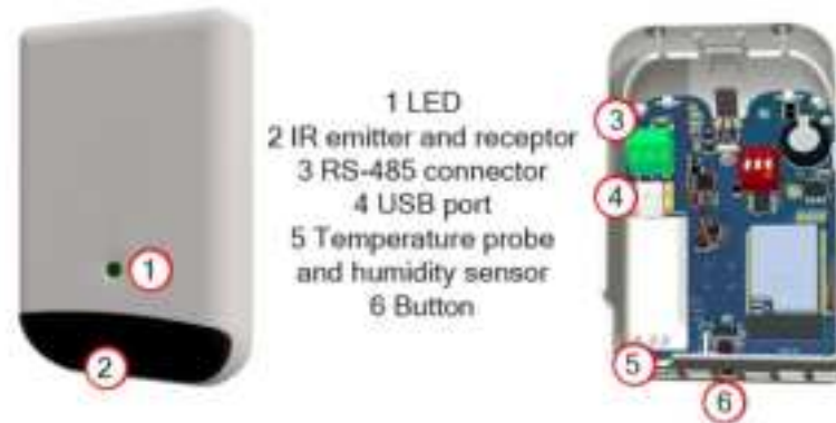
Figure 3.4 Built-in ports and sensors.
