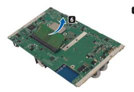
Pull out the memory module from the socket.
