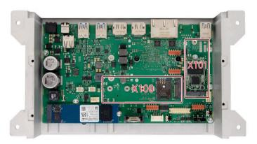
Siemens IPCs provide the standardized openings in the housing to extend the devices with additional external interfaces.
