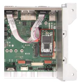
Align the golden finger on the M.2 Module on your mother-board, and then press firmly until the M.2 Module is completely seated on the slot.
