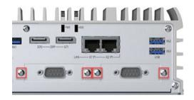
Unscrew either one set of the marked screws for fixing the COM interface.
