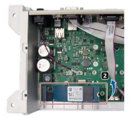
Align the golden finger on the M.2 NVMe/SATA SSD to the motherboard, then press firmly until the M.2 NVMe/SATA SSD is completely seated on the slot.
