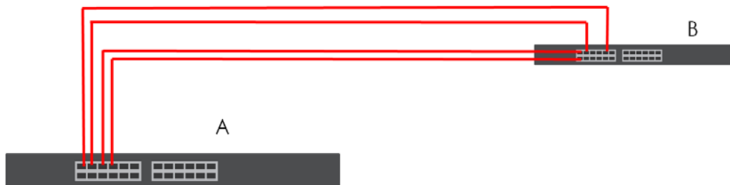
Figure 165 Trunking Example – Physical Connections
