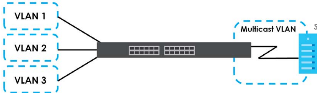
Figure 200 MVR Network Example
