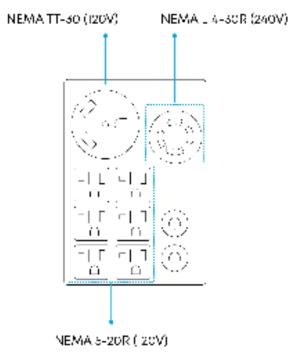
If the six 120V sockets at the bottom have no devices connected and the two 240V sockets at the top draw less than 20W, the AC output will automatically turn off after 15 minutes. This can happen with intermittently working devices like refrigerators or pumps.
