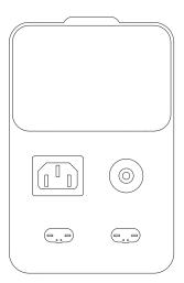
Each solar input port supports a voltage range of 11-165V, a maximum current of 17A, and a maximum input of 1,600W. With two ports, the system can handle up to 3,200W in total. Ensure that the total voltage of connected solar panels does not exceed the 165V for each solar input, as this may cause damage to the product or to the solar panels themselves.
