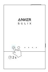
b. After powering on, confirm the indicator light is in the upper left as shown.
