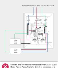
If the PE and N wires are transposed when Anker SOLIX Home Power Panel/Transfer Switch is connected to a subpanel, the 120V load wire may become damaged.
