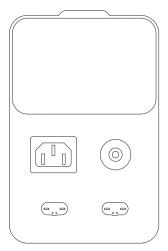
Each solar input port supports a voltage range of 11-165V, a maximum current of 17A, and a maximum input of 1,600W. With two ports, the system can handle up to 3,200W in total. Ensure that the total voltage of connected solar panels does not exceed the 165V for each solar input, as this may cause damage to the product or to the solar panels themselves.
