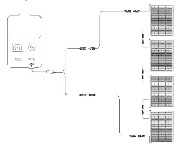
• Supports a 2S2P (2 in series, 2 in parallel) configuration. For example, review this image showing Anker SOLIX 400W Portable Solar Panels (48V/8.3A).
