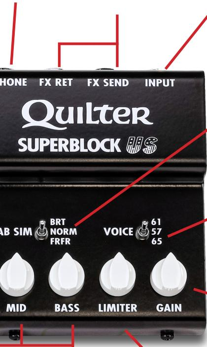
**CAB SIM:** operates on the signal going to the HEADPHONE and LINE OUT jacks. FRFR presents a flat full range signal suitable for external cab-sim models. NORM engages an internal cab sim that represents a normal 12-inch guitar speaker, and warms up the sound for headphones and direct console outputs. BRT increases treble response to represent small bright guitar speakers.
