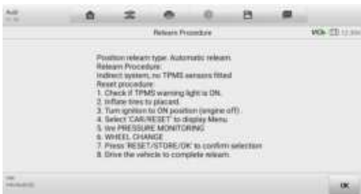
Figure 5-13 Relearn Procedure for Indirect TPMS
