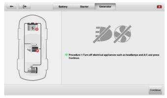
Figure 7-11 Generator Test Screen
