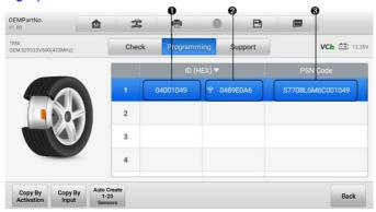
Figure 5-35 Programming Screen via OEM Part NO.
