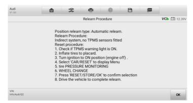
Figure 5-13 Relearn Procedure for Indirect TPMS
