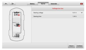
Figure 7-10 Starter Test Result Screen
