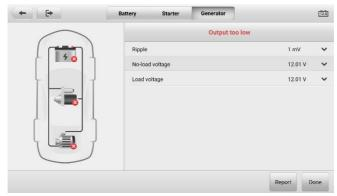
Figure 7-12 Generator Test Result Screen
