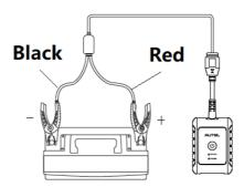
Figure 7-2 Connecting to a Battery
