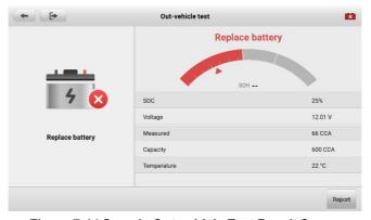
Figure 7-14 Sample Out-vehicle Test Result Screen
