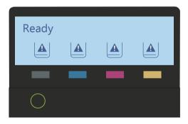
When you install the cartridge, the printer displays "Ready". The cartridge chip is recycled and it will show icon, but it will NOT affect printing, so you can start to print.
