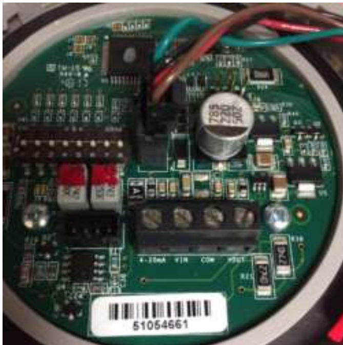
FIGURE 38 8301-067 Sensor Dip Switches
