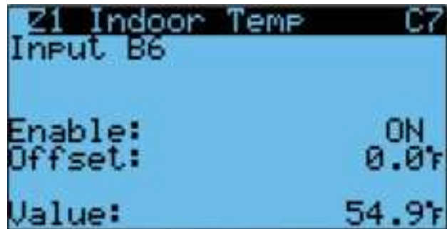
FIGURE 37 Enable/Disable Zone 1 Indoor Temperature Sensor
