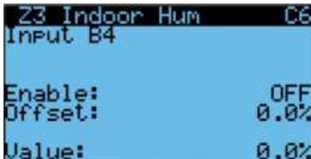
FIGURE 36 Enable/Disable Zone 3 Indoor Humidity Sensor
