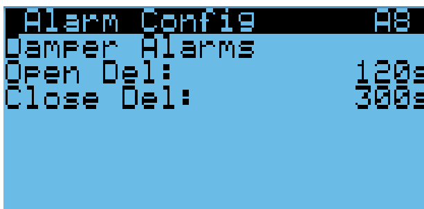
FIGURE 17 Adjusting Damper Alarm Values
