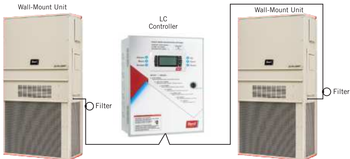
FIGURE 19 Communication Wiring (Alternate Method)
