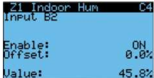
FIGURE 33 Enable/Disable Zone 1 Indoor Humidity Sensor
