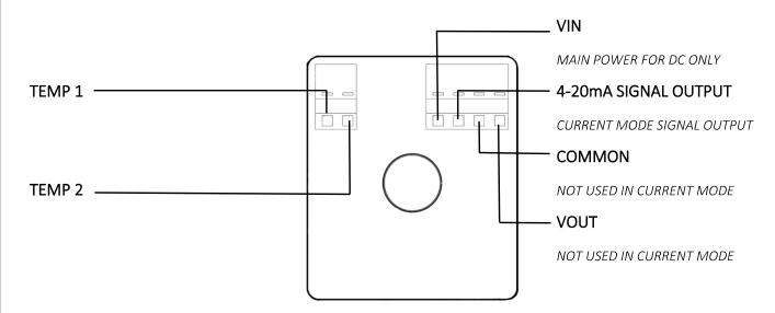
Temp Element: Interchangeable NTC thermistor, 2-wire
