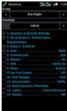
Electronic checklist capability keeps cockpit paperwork to a minimum
