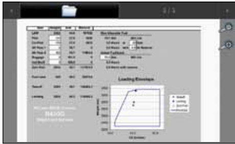
Electronic flight bag functions can display Weight & Balance documents
