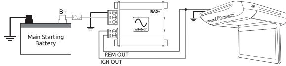
Note: If setting any turn-on or turn-off delays, make sure to apply the same delays to both IGN OUT and REM OUT.
