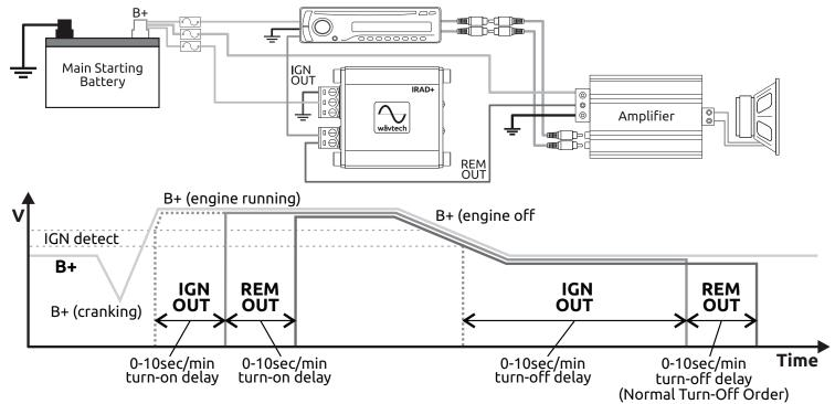
**Notes:** This is just one of many applications for generated outputs with linked delays, where in normal turn-off order REM OUT follows IGN OUT delays based upon engine running status. The additional settings available are:
