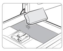
**4.** If the items are heavily soiled, pour a small amount of detergent onto the door for better cleaning results.
