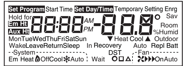
Fig. 8. Display of all the segments of the LCD.
