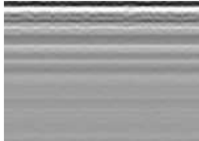
Bad Skyshot: horizontal bands are present in the GPR Imagery when the detector is still raised.
