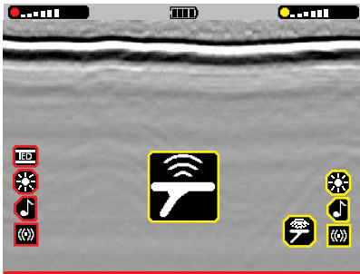
Bad Skyshot: horizontal bands are present in the GPR Imagery when the detector is still raised.
