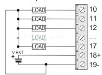
The digital outputs must be powered externally to function properly (V EXT).
