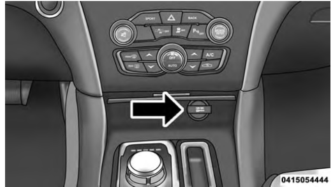
Front Power Outlet
