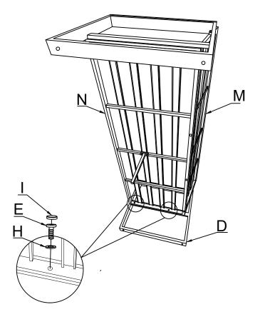
Do not fully tighten all bolts until assembly is complete.
