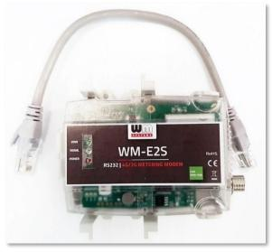
Step #8: Ensure that the internal antenna U.FL - black - cable is connected to the U.FL connector (9)!
