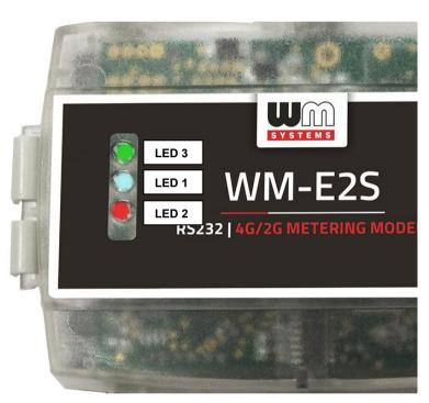
At the first power on - during the charge – the **green** LED is flashing quickly. After a few minutes the LED will be blank, then qill be flashing quickly again. When the **green** LED will be flashing slowly and the other LEDs will be lighting according the NORMAL operation, then the modem will be charged completely and it will be ready for congfiuring and to operate.
