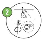
Mark the locations to install the 2 screws. Carefully drive screws in, leaving a little over a 1/16" gap.
