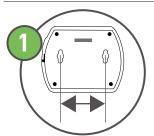
Locate the sites for the screws by measuring the distance from the centre from one keyhole slot to the other.
