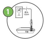
Before first use, use the micro USB cable (included) to charge the product until the indicator light turns green.
