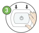
Slide the product's two keyhole slots over the two screw heads until both sides are captured by the narrow end of the keyhole slots.
