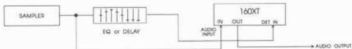
Figure 9: Using the 160XT with a Sampler
