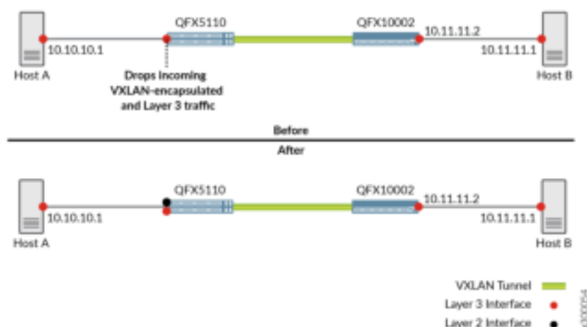
Figure 52: Results When Routing Traffic Between a VXLAN and a Layer 3 Logical Interface Is Disabled (Before) and Enabled (After)
