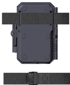
Figure 17: Mounting the Camera
