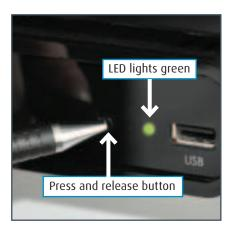
Briefly press (1 second) and release the SYNC/update button on the front of the Control Box. The Status LED will illuminate green.
