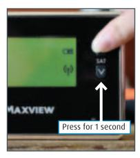
Press Satellite UP or Down button on the panel to pair.
