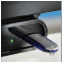
**3.** Insert the USB flash memory stick. The SYNC LED will flash GREEN whilst data is being transferred.
