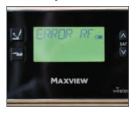
The Control Panel will read ERROR RF so you will need to pair the Control Panel and Control Box.
