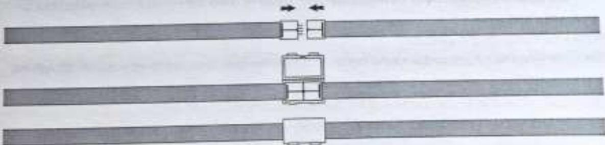
To extend the lightstrip, please purchase Yeelight Lightstrip Plus Extension. Match the end of original lightstrip with the connection port of Lightstrip Plus Extension and put into fastener. Be sure each strip is tightly connected to the other before continuing to mount the next strip. The max. extension is 10 metres.
