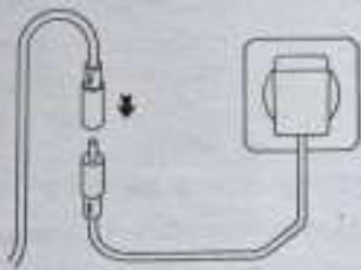
Connect and plug in the power supply.
