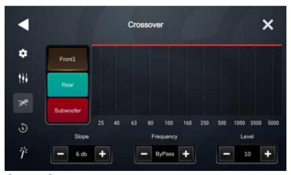
[Crossover]: You can adjust Slope, Frequency, Level of these parameters
