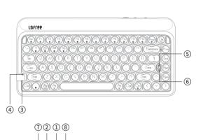
Mode Switch WLS: Bluetooth Mode /2.4G Mode OFF: Power Off CAB: Wired Mode ② System Switch
