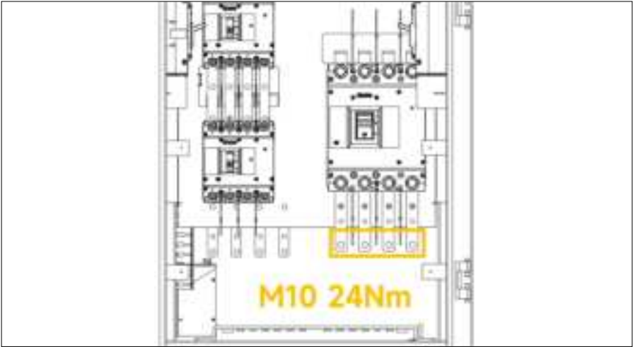
Figure 5. grid side - copper busbar terminal connection
