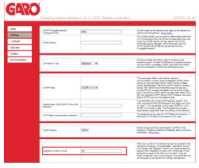
**3.** On bottom of the screen, click "**Save & Restart**" to save the configuration. Once the controller has been restarted the operator current limit should be set, and you can now try a charging session to confirm.
