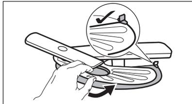
7. Reassemble the filters (B) and (C).
