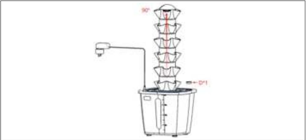
Figure 8: The water storage bucket is poured into the 20 liter nutrition solution with a folding funnel, the water inlet nozzle is covered, the intelligent switch is inserted into the power supply, and the balance of the foot is adjusted to 90° so that each layer of the water tower has the nutrient solution flowing through, then it can be used normally.
