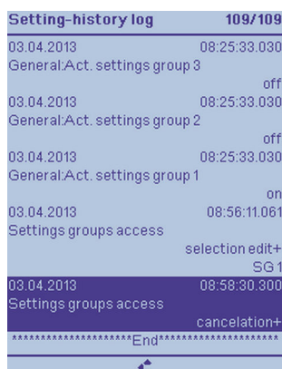
Figure 3-7 Reading the Setting-History Log on the On-Site Operation Panel of the Device
