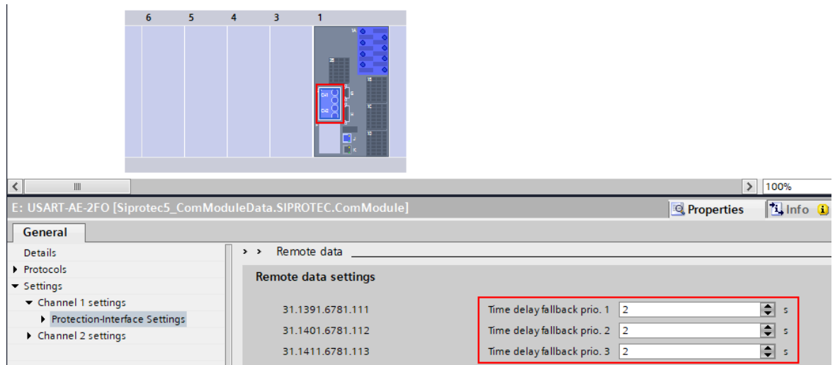
Figure 3-71 Parameterization of Dropout Time for Signals of Different Priorities
