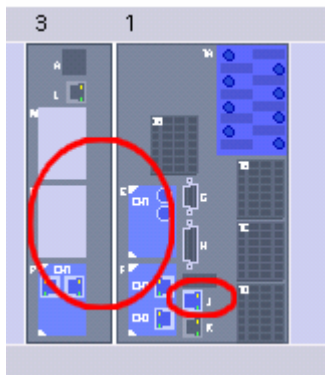
Figure 5-41 Inserting an Ethernet Module
