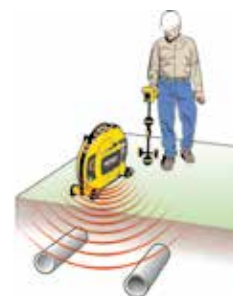
Induce a signal to locate utilities.
