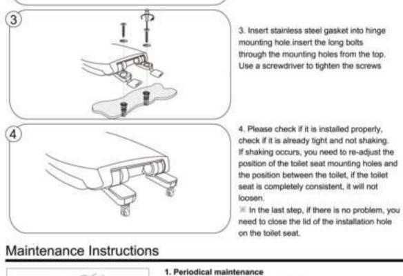
4. Please check if it is installed properly, check if it is already tight and not shaking. If shaking occurs, you need to re-adjust the position of the toilet seat mounting holes and the position between the toilet, if the toilet seat is completely consistent, it will not
