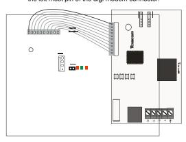
Programming requirements for the COM unit can be found in the *Premier Elite* installation manual INS176.The red lead should be positioned on the uppermost pin of the COM unit.
