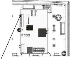
The red lead should be positioned on the uppermost pin of the COM unit.
