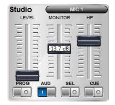
In the Studio Monitoring section, also a Talkback section is provided and consists of four buttons and the "LEVEL" control. This section allows for direct conversation with the studio monitors, headphones, telephone hybrid 1 or telephone hybrid 2.
