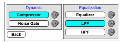
In order to activate/deactivate a process, just click on the button with its name. When the process is active, it will appear with a blue background, otherwise the button will have white background.
