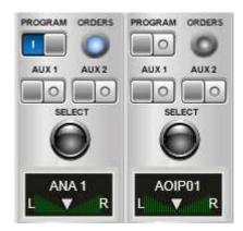
If the channel has an output channel assigned in the "Orders" field, when you press the "ORDERS" button it will turn on (see image on the right) and the orders microphone will be sent to that output. Just like on the console control surface, the operation of that button is in PTT mode.
