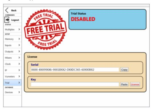
You must "Copy" the "Serial" code by means of the associated button and send it to AEQ in order to generate the associated "Key" and send it back to you (you must "Paste" it by means of the associated button).
