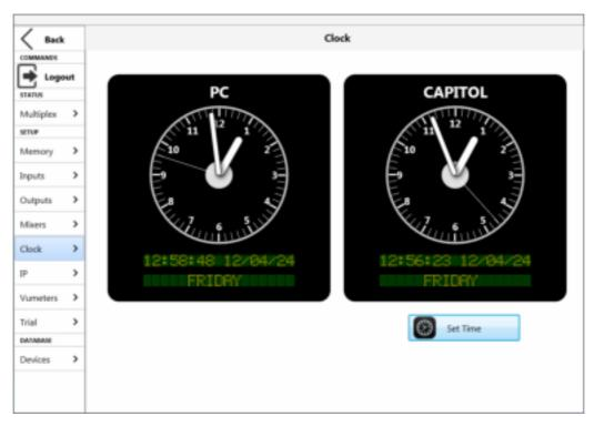
By clicking on the "**Set Time**" button, console time is synchronized to the device's time. For Windows version, the leftmost clock will be labeled "PC" while for iOS versions it will say "iPad".
