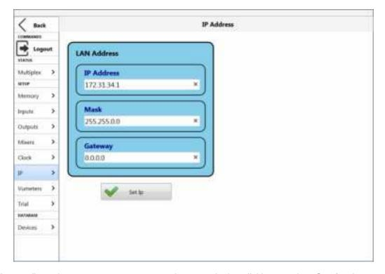
The configured parameters are sent to the console by clicking on the "Set Ip" button. A message indicates that these changes will not be active until you turn off and on the console.
