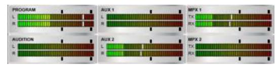
The "PROGRAM" and "AUDITION" vumeters are always displayed, whereas the rest of them are only shown when no channel is selected by means of the button
