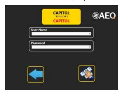
If the "Auto Login" option is configured in the devices section (for the selected device), this screen will appear only temporarily, and as soon as all the configuration data is received from the console, it will give pass to next screen. On the other hand, if that option is not activated, the user must type in a valid user and password to continue.
