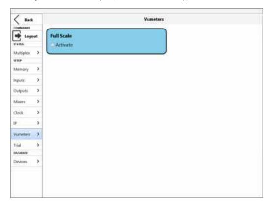
The "Full Scale" option allows you to activate the vumeters display in dBFs (0dBFs = +24dBu).
