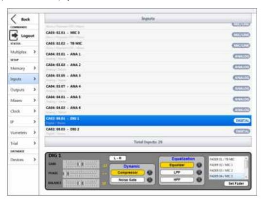
For each input, virtual module type (for example, digital CA02 or hybrid CA33), virtual slot number (for example, 06), channel number within that virtual slot (for instance, 01), input's logic name (for example, DIG 1), signal type (for example, DIGITAL) and configuration details (for example, Digital / Stereo) are displayed.
