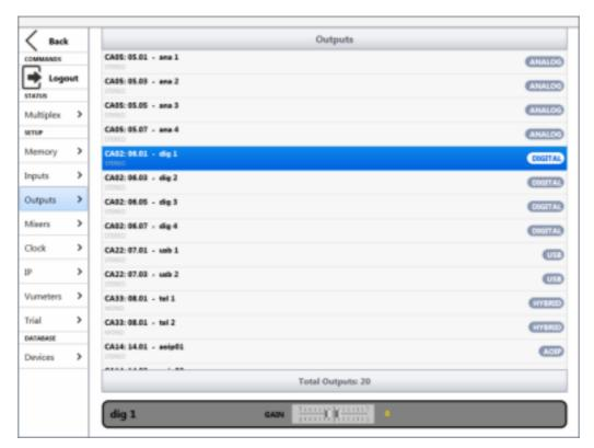
For each output, virtual module type (for example, digital CA02 or hybrid CA33), virtual slot number (for example, 06), channel number within that virtual slot (for instance, 01), output's logic name (for example, dig 1), signal type (for example, DIGITAL) and signal channels number (for example, STEREO) are displayed.
