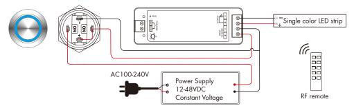
• Connect with push switch panel, negative trigger input. Press the panel to switch or adjust brightness.
