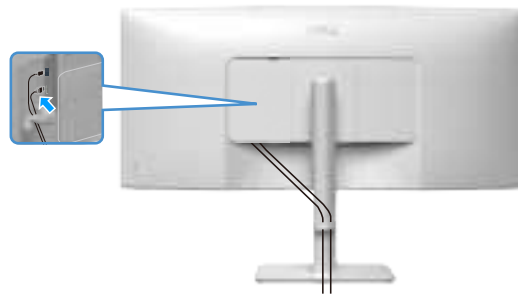
Figure 22. Attaching the side I/O-cover
