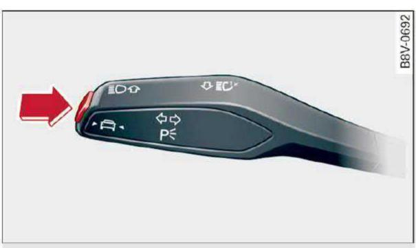
Fig. 119 Turn signal lever: button for Audi active lane assist
