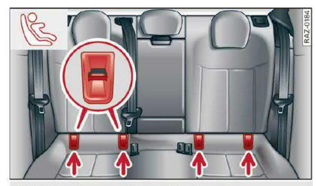
Fig. 70 Rear bench seat: lower LATCH anchors
