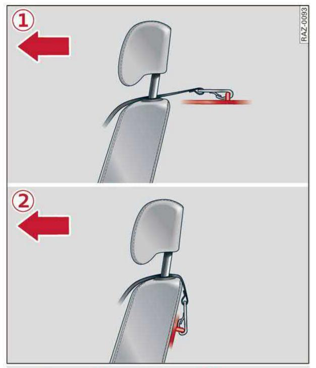
Fig. 72 Version 1 rear shelf / Version 2 rear backrest: securing the upper strap on the top tether anchor
