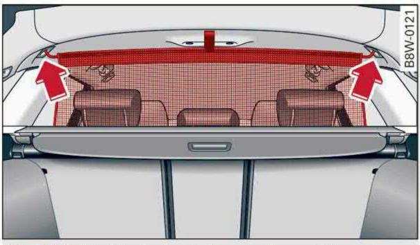
Fig. 81 Behind the backrest: hanging the partition net
