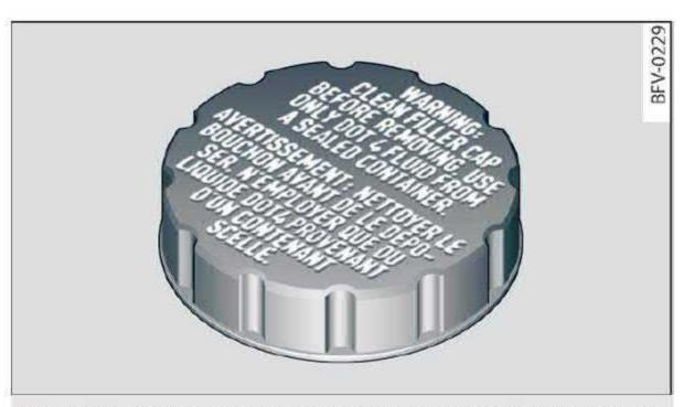
Fig. 162 Engine compartment: cap on brake fluid reservoir
