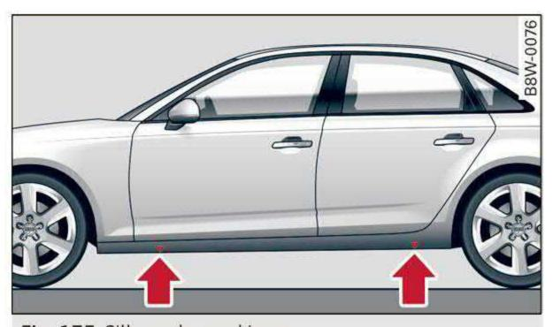
Fig. 175 Sill panels: markings
