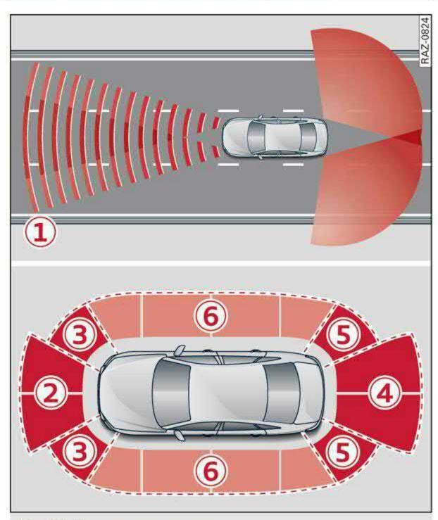
Fig. 99 Sensor coverage area
