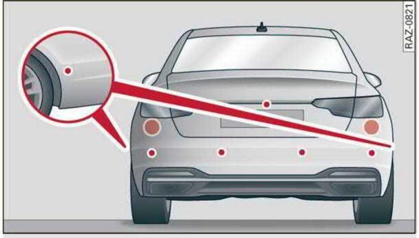
Fig. 102 Rear area: sensors and cameras
