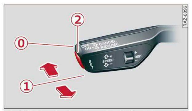
Fig. 109 Operating lever: operating adaptive cruise control
