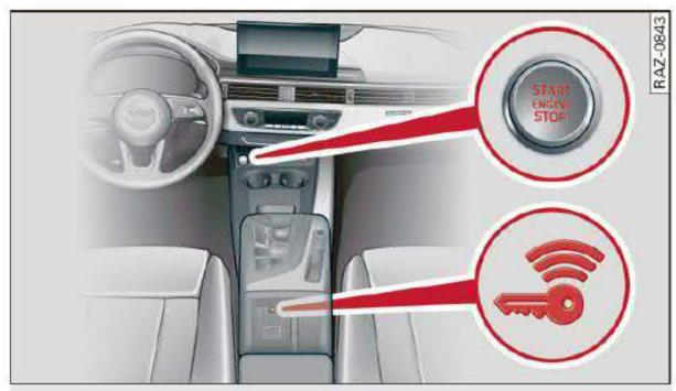
Fig. 93 Center console: starting the engine
