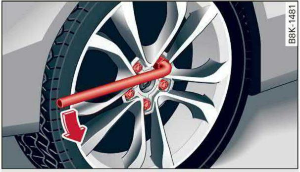
Fig. 174 Wheel: loosening the wheel bolts
