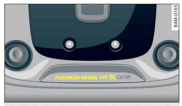
**Fig. 69** Headliner: indicator light to display the status of the front passenger's airbag
