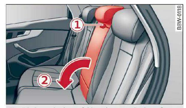
Fig. 78 Center backrest: folding the center backrest forward
