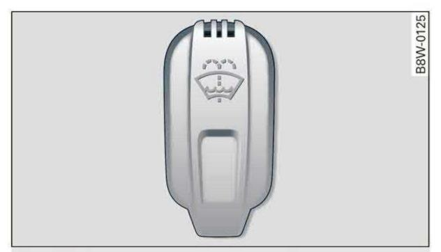
Fig. 164 Engine compartment: washer fluid reservoir cap
