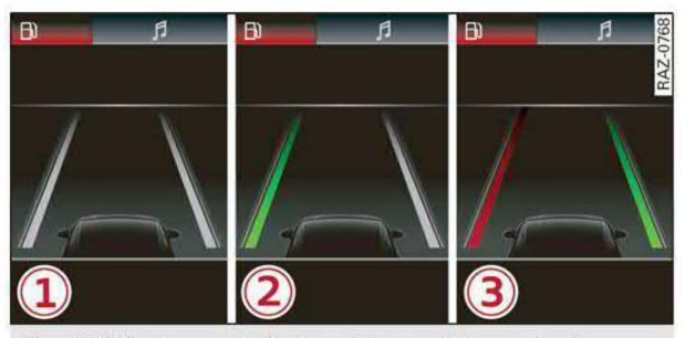
Fig. 118 Instrument cluster: driver assistance display
