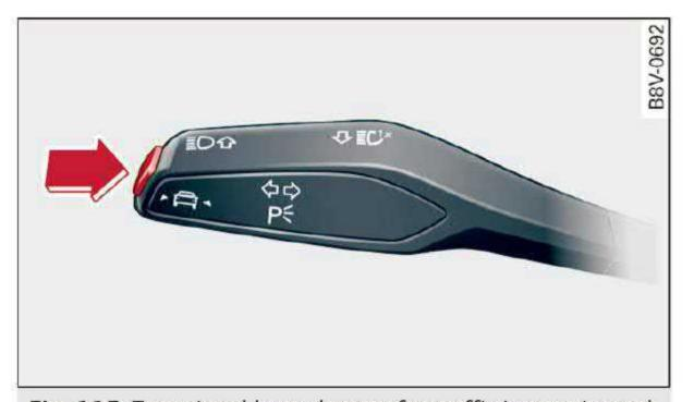
Fig. 115 Turn signal lever: button for traffic jam assist and Audi active lane assist
