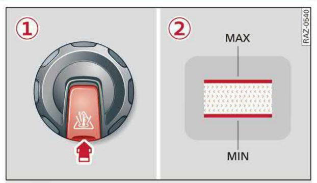
Fig. 161 Engine compartment - Coolant expansion tank:
