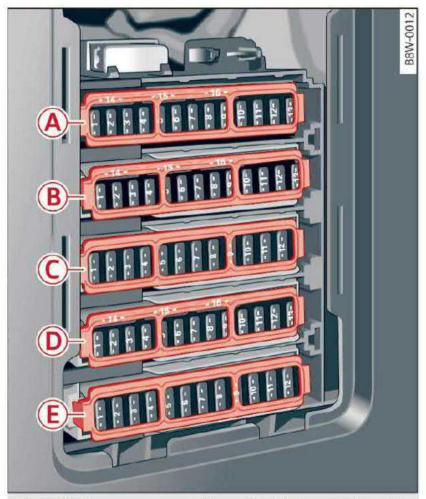
Fig. 185 Front passenger's footwell (right-hand drive vehicle): fuse panel with plastic clip
