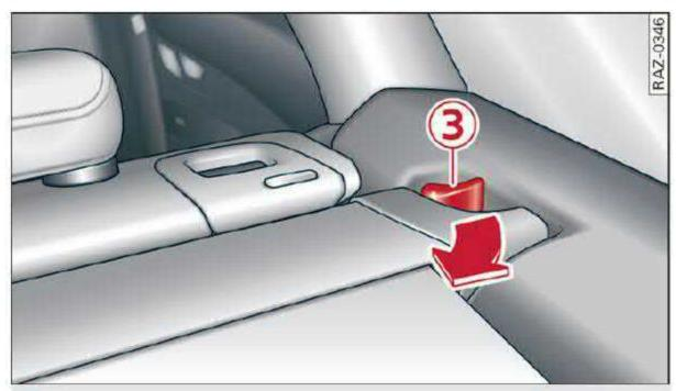
**Fig. 76** Luggage compartment: removing the luggage compartment cover
