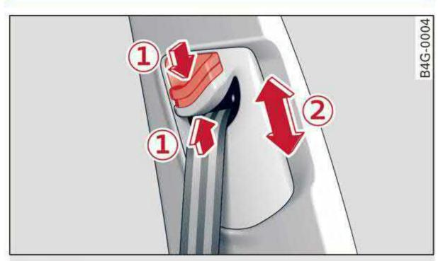
Fig. 67 Belt height adjustment for the front seats - safety belt relay
