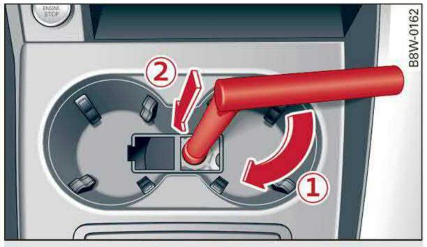
Fig. 98 Front cup holder: parking lock emergency release
