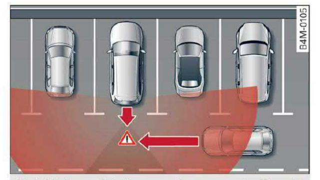
Fig. 129 Sensor detection range for rear cross-traffic assist
