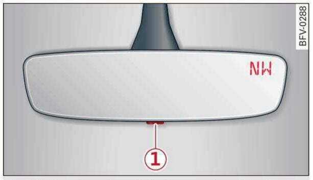
Fig. 54 Rearview mirror: digital compass is switched on
