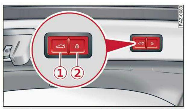
Fig. 31 Luggage compartment lid: 1 closing button\*, 2 lock button\* (vehicles with convenience key\*)
