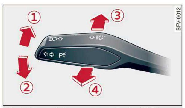
Fig. 42 Lever: switching on the turn signal and high beams
