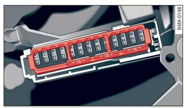
Fig. 186 Driver side cockpit: fuse panel with plastic bracket
