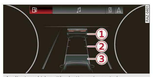
Applies to: vehicles with adaptive cruise control: **Fig. 116** Instrument cluster: display of the current distance
