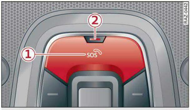
Fig. 137 Front headliner: cover for the emergency call but-
