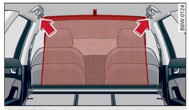
Fig. 84 Folded backrest: setting up the partition net
