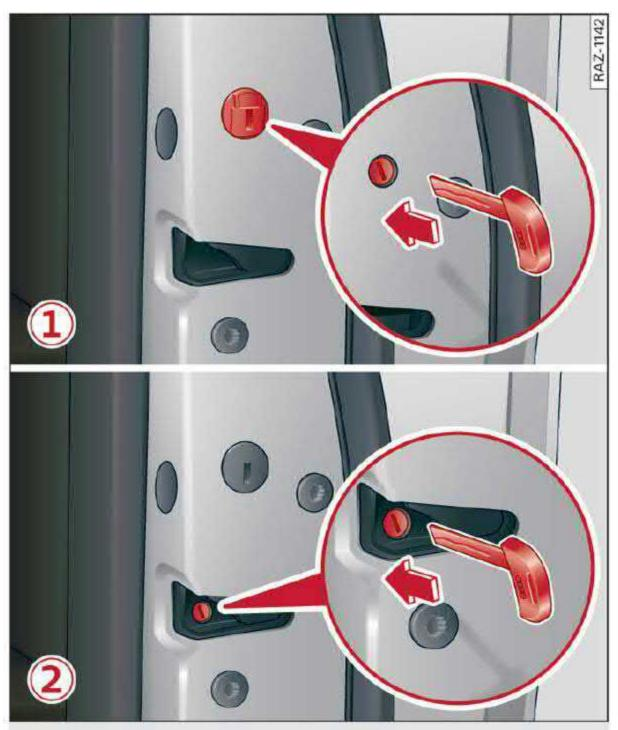
Fig. 25 Door: mechanically locking
