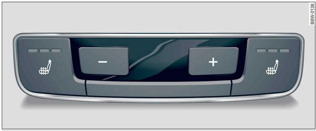
Fig. 92 3-zone deluxe automatic climate control system: rear controls
