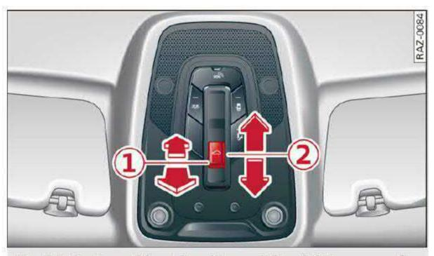
Fig. 39 Section of front headliner: sliding/tilting sunroof button
