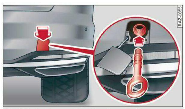
Fig. 181 Rear bumper: installing the towing loop
