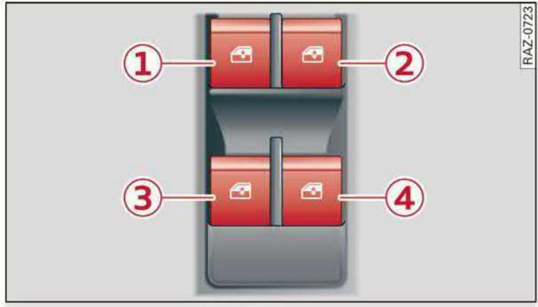
Fig. 38 Driver's door: power window switch
