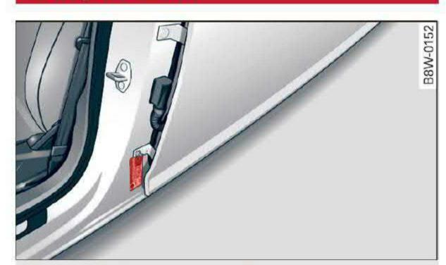
Fig. 167 Driver's side B-pillar: tire pressure label
