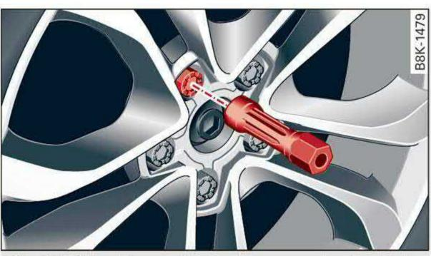
Fig. 177 Wheel: internal hex socket to turn the wheel bolts
