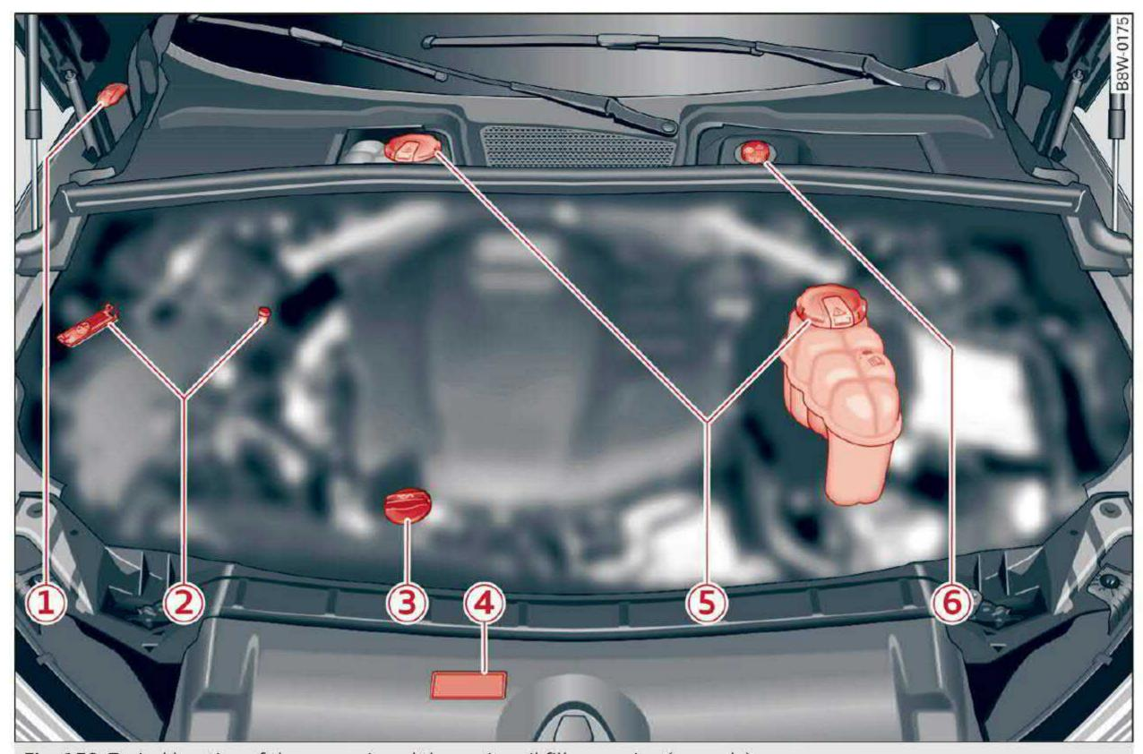
Fig. 159 Typical location of the reservoir and the engine oil filler opening (example)
