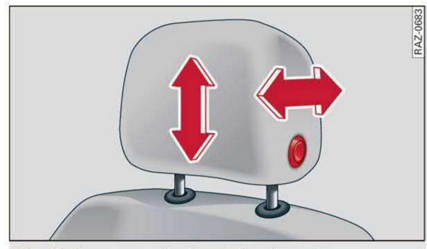
Fig. 61 Front seat: adjusting the head restraint
