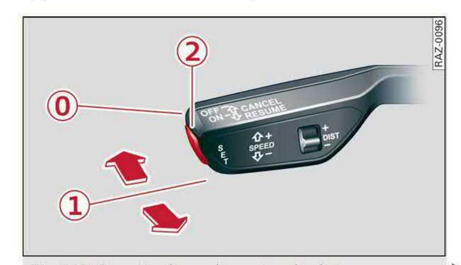
Fig. 112 Operating lever: decreasing the distance
