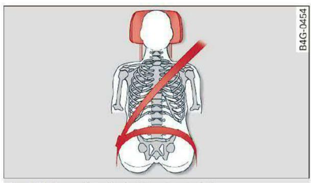
Fig. 60 Correctly-adjusted head restraint
