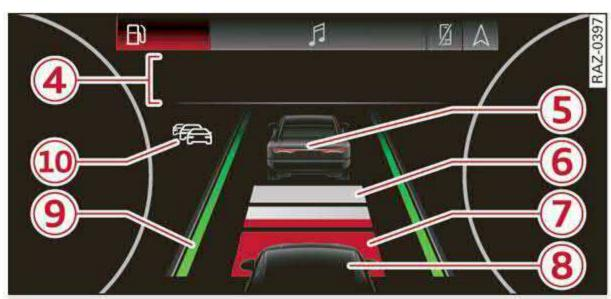
Fig. 108 Instrument cluster: driver assistance display
