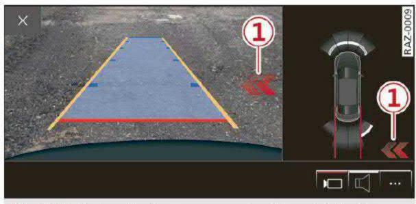
Fig. 130 Center display: rear cross-traffic assist display
