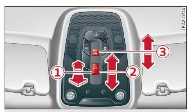
Fig. 40 Headliner: panoramic glass roof and sunshade\* buttons
