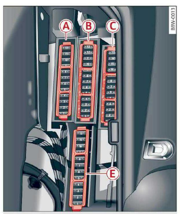
Fig. 187 Left side of the luggage compartment: fuse panel with plastic clip
