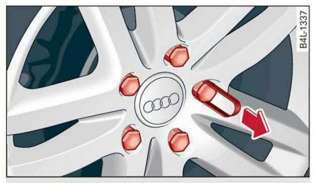
Fig. 173 Wheel: wheel bolts with caps
