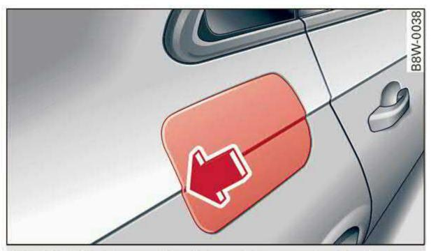
Fig. 153 Right rear side of the vehicle: opening the fuel filler door
