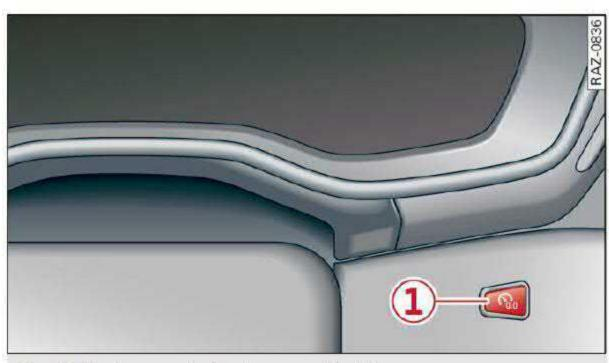
Fig. 7 Instrument cluster: reset button
