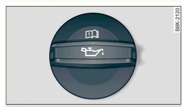
Fig. 160 Engine compartment: engine oil filler opening cover
