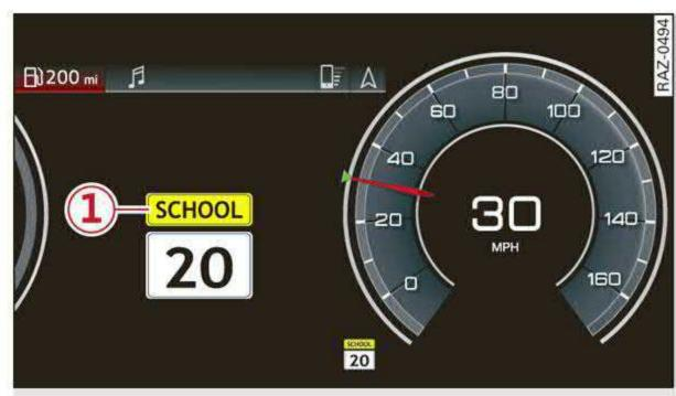
Fig. 103 Instrument cluster: traffic sign recognition
