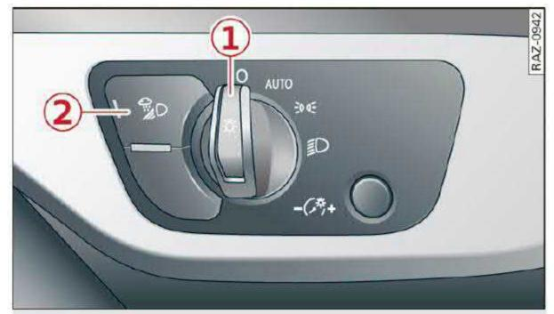
Fig. 41 Instrument panel: light switch with button
