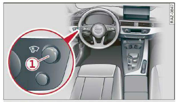
Fig. 19 Instrument panel: knob for the head-up display
