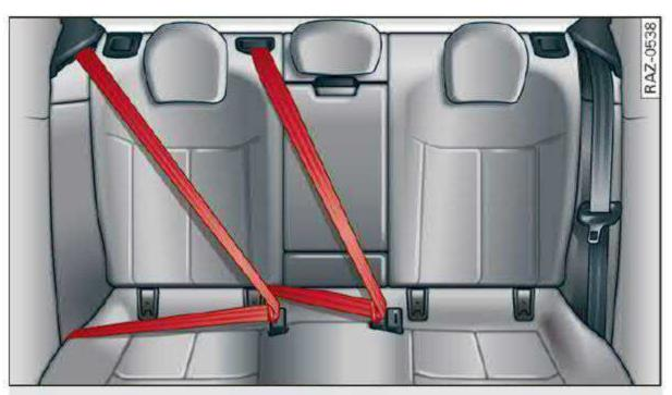
Fig. 73 Rear bench seat: securing unused safety belts
