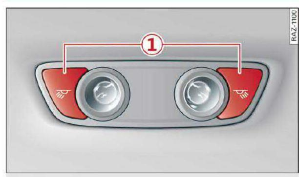
Fig. 45 Headliner: rear reading lights
