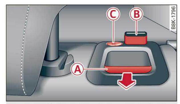
Fig. 77 Outer backrest: release lever, securing knob, and lock\*
