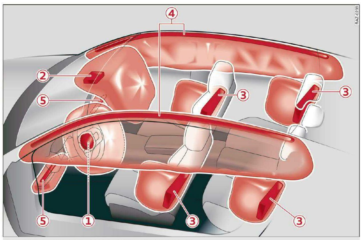
Fig. 68 Airbag overview image (enlarged section: deployed airbags)
