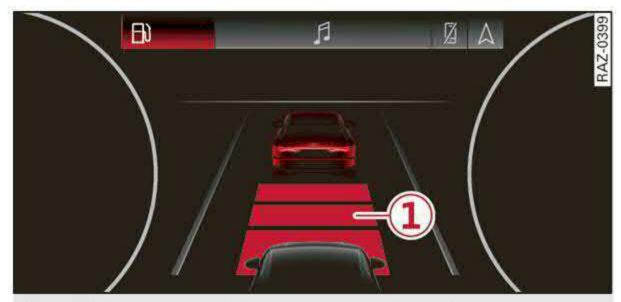
Fig. 114 Instrument cluster: request for driver intervention
