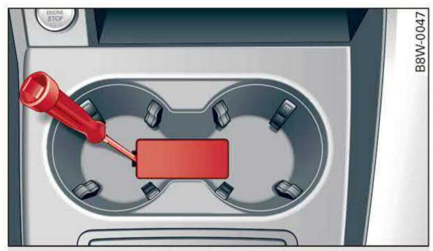
Fig. 97 Front cup holder: removing the cover
