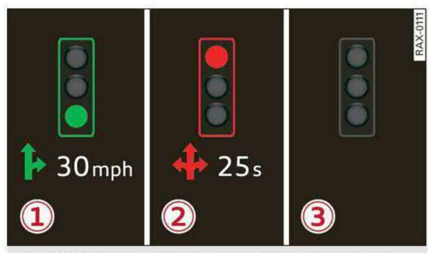
Fig. 104 Instrument cluster: traffic light information display
