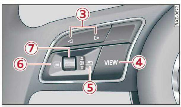
Fig. 5 Left side of multifunction steering wheel
