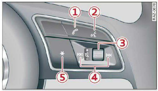
Fig. 21 Right side of the multifunction steering wheel
