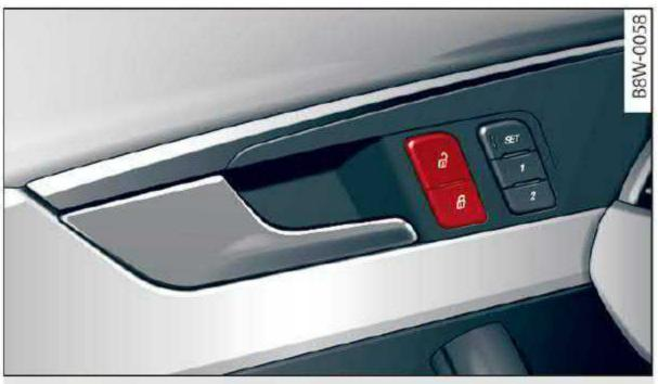
Fig. 23 Driver's door: central locking switch
