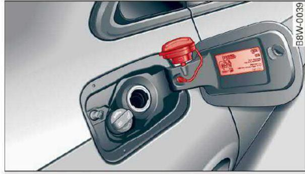
Fig. 154 Fuel filler door with attached fuel cap
