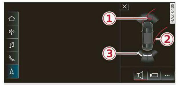
Fig. 124 Center display: distance display
