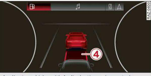
Applies to: vehicles with Audi adaptive cruise control Fig. 117 Instrument cluster: distance warning
