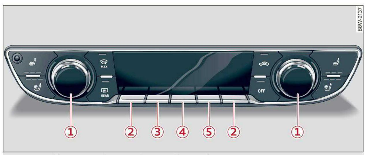
Fig. 91 3-zone deluxe automatic climate control system: cockpit controls
