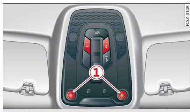
Fig. 44 Headliner: front interior lighting
