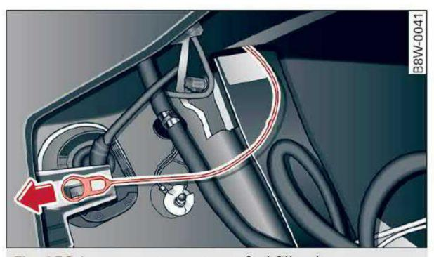
Fig. 156 Luggage compartment: fuel filler door emergency release
