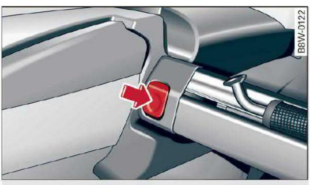
Fig. 82 Behind the backrest: removing the partition net
