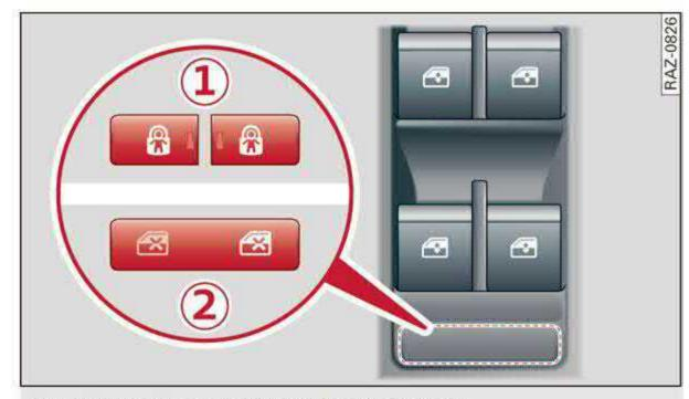
Fig. 36 Section of driver's door: controls
