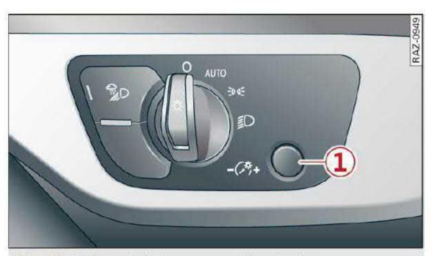
Fig. 46 Light switch: instrument illumination
