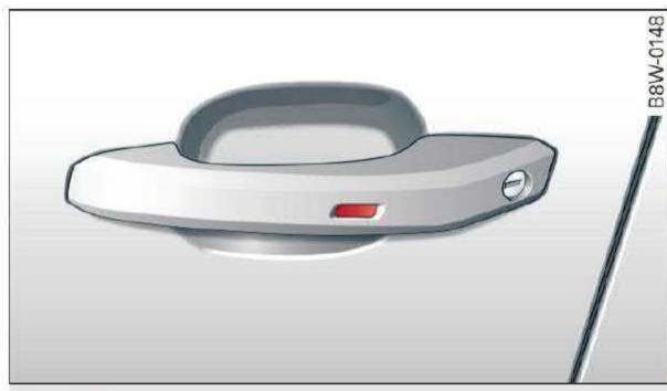
Fig. 27 Door handle: sensor for locking
