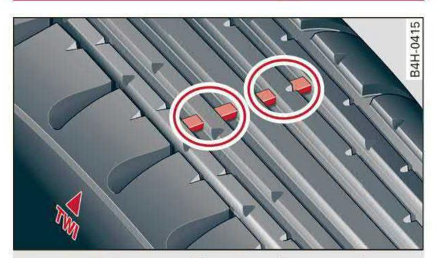
Fig. 166 Tire profile: treadwear indicator
