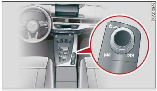
Fig. 22 MMI On/Off knob with joystick function
