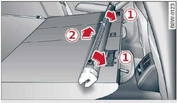
Fig. 83 Folded backrest: installing the partition net
