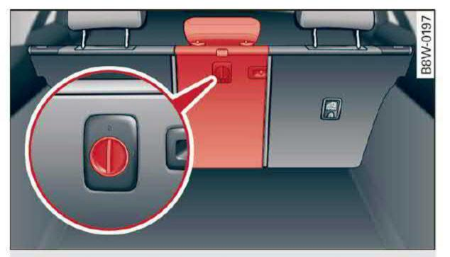
Fig. 80 Center backrest: pass-through release
