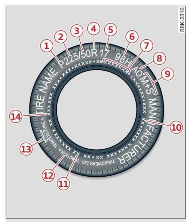
Fig. 165 Tire designations on the sidewall
