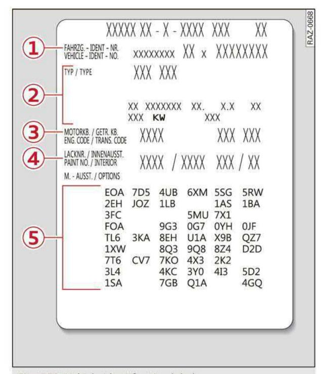
Fig. 189 Vehicle identification label
