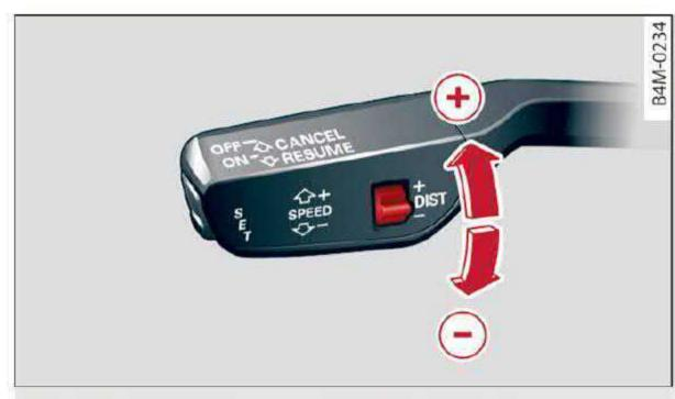
Fig. 111 Operating lever: setting the distance
