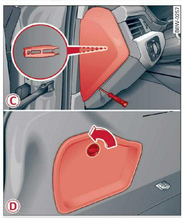
Fig. 183 Driver's side cockpit (left-hand drive/right-hand drive vehicles): cover ©, left side of luggage compartment: cover ©
