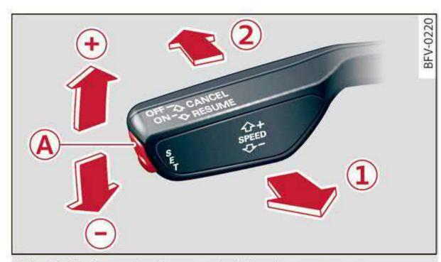
Fig. 105 Operating lever: switching the system on
