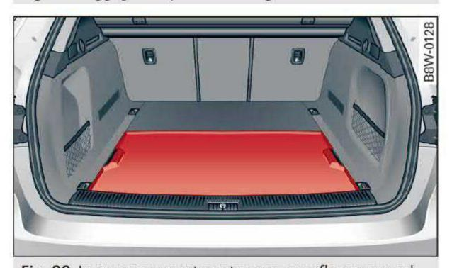
Fig. 88 Luggage compartment: cargo area floor reversed
