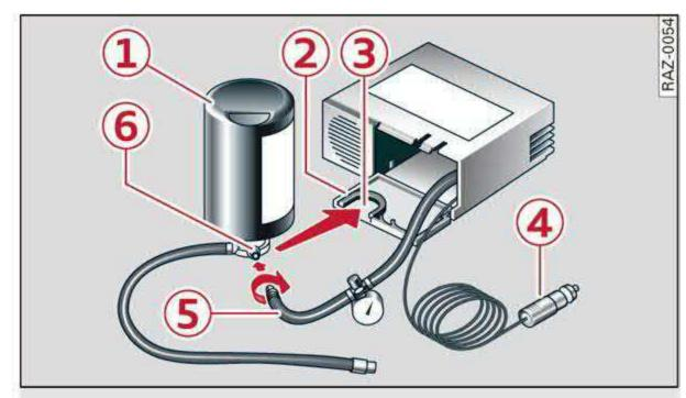
Fig. 171 Components of the tire mobility kit
