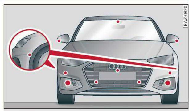
Fig. 101 Front area: sensors and cameras
