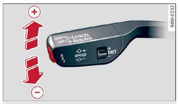
Fig. 110 Operating lever: changing the speed
