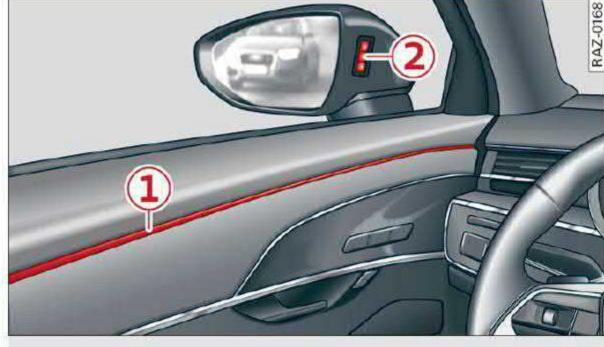
Fig. 122 Front door: exit warning
