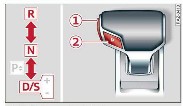
Fig. 94 Center console: selector lever
