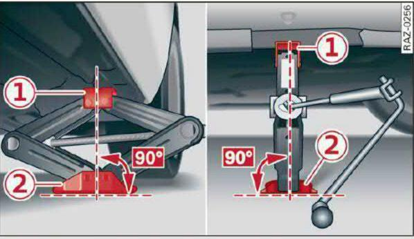
Fig. 176 Sill: positioning the vehicle jack
