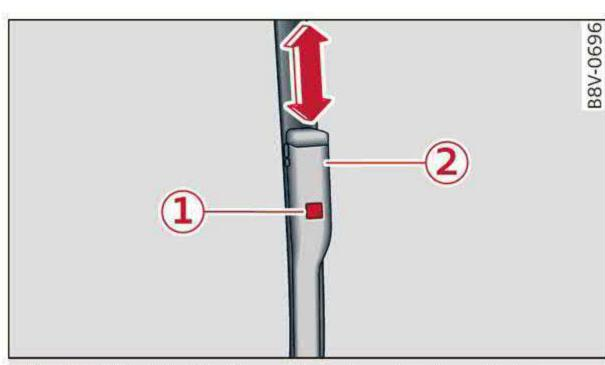
Fig. 52 Windshield wipers: changing the wiper blades
