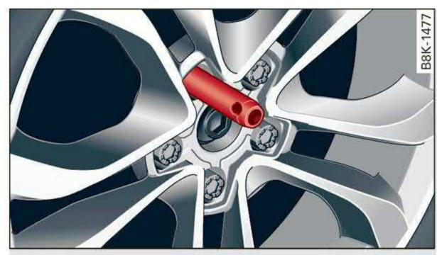
Fig. 178 Wheel: alignment pin in the top hole
