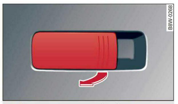
Fig. 79 Luggage compartment: release lever
