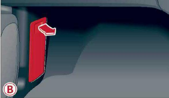
Fig. 182 Driver's side footwell (left-hand drive vehicles): footrest (A), front passenger's footwell (right-hand drive vehicles): cover (B)
