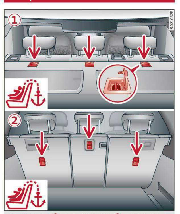
Fig. 71 Version ① rear shelf / Version ② rear backrest: top tether anchors for securing a child safety seat with an upper strap
