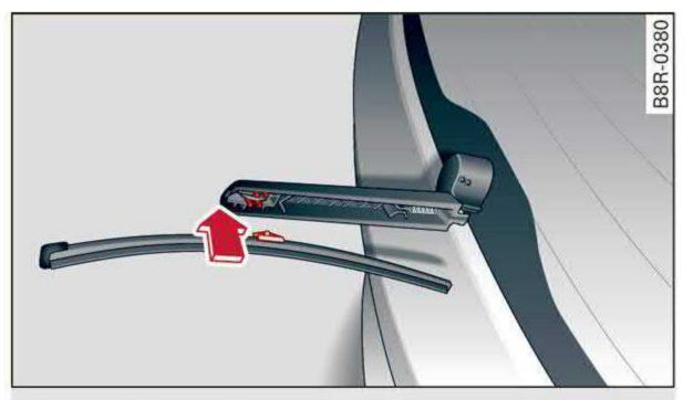
Fig. 53 Rear window wiper: installing the wiper blade
