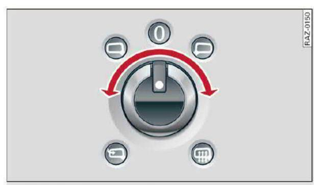
Fig. 47 Driver's door: knob for the exterior mirrors
