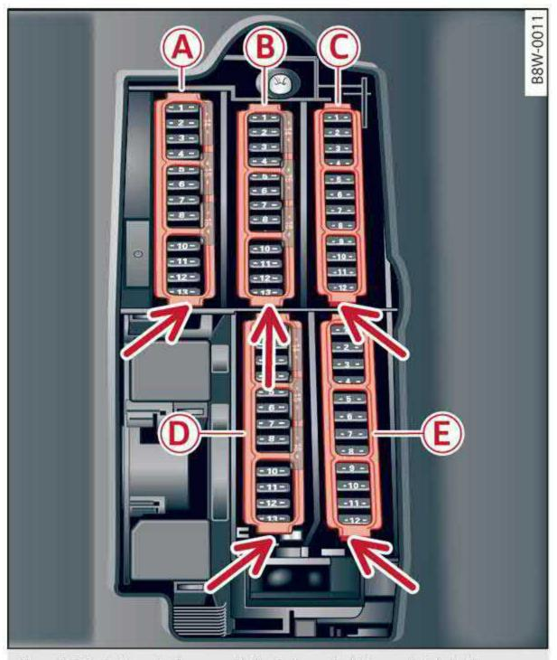
Fig. 184 Driver's footwell (left-hand drive vehicle): fuse panel with plastic clip
