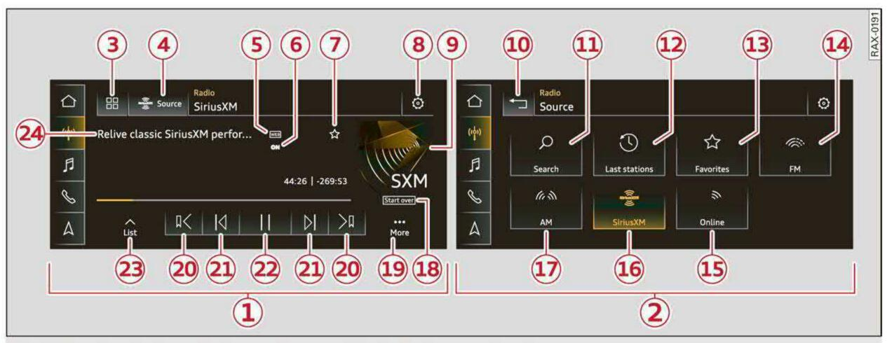
Fig. 149 Center display: left side: playback view of radio functions, right side: sources
