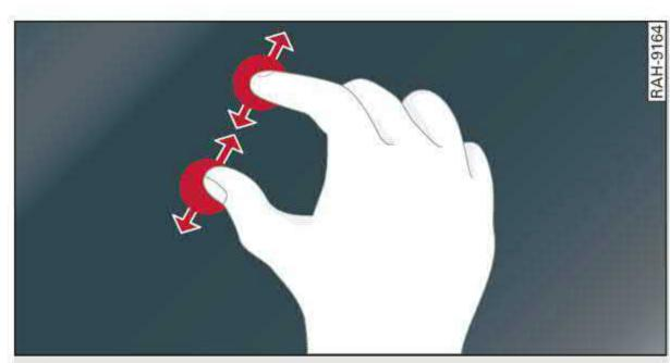
Fig. 11 Touch display: pinching fingers together and pulling them apart
