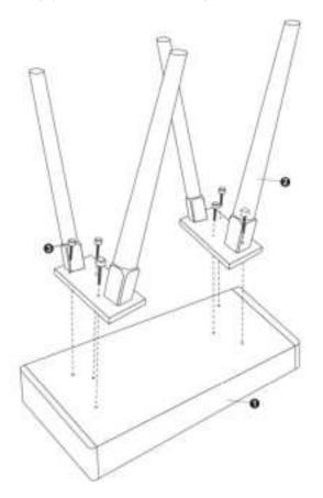
Securely fasten the mounting plates with the assembled support legs (2) to the console using the six plastic head screws (3).
