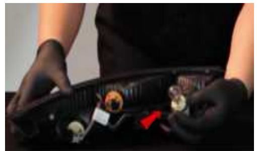
4. Remove fog lamp bulb from socket. (Never touch bulbs with bare hands)
