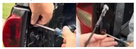
**2.**Remove the original factory taillight assembly, and all taillight sockets and bulbs(Note: The original reversing lights need to be retained and installed on the new lights).
