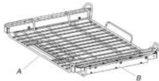
A. SatinGlide™ roll-out extension rack for Smart Oven+ Attachments B. Sliding shelf
