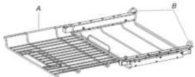
A. SatinGlide™ roll-out extension rack for Smart Oven+ Attachments B. Sliding shelf
